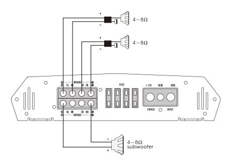
system 3: 2channel bridged connection
